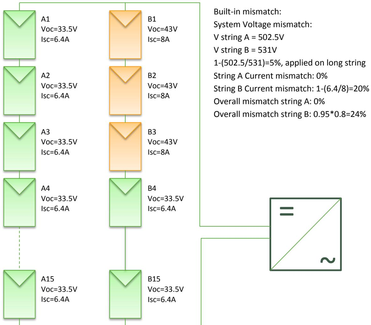
Notice that this example also demonstrates that the power variation between the different modules has no restrictions. As long as current and voltage variations obey the 25% rule, you can mix and match modules with any power rating or technology available: Mono-crystalline, Multi-crystalline and even Thin-film.
