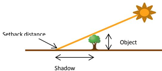
The annual energy production of a PV system in San Francisco was modeled with different setback ratios. The percentage of hours per year impacted by shading is shown in Figure 1. With a setback ratio of 1.5, 14% of annual hours are impacted. Increasing the setback ratio reduces the amount of annual affected hours dramatically.
