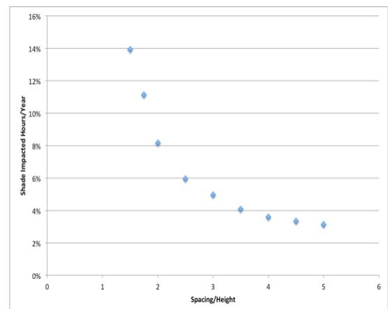
Figure 1: The Effect of Shade—Without Tigo Energy
